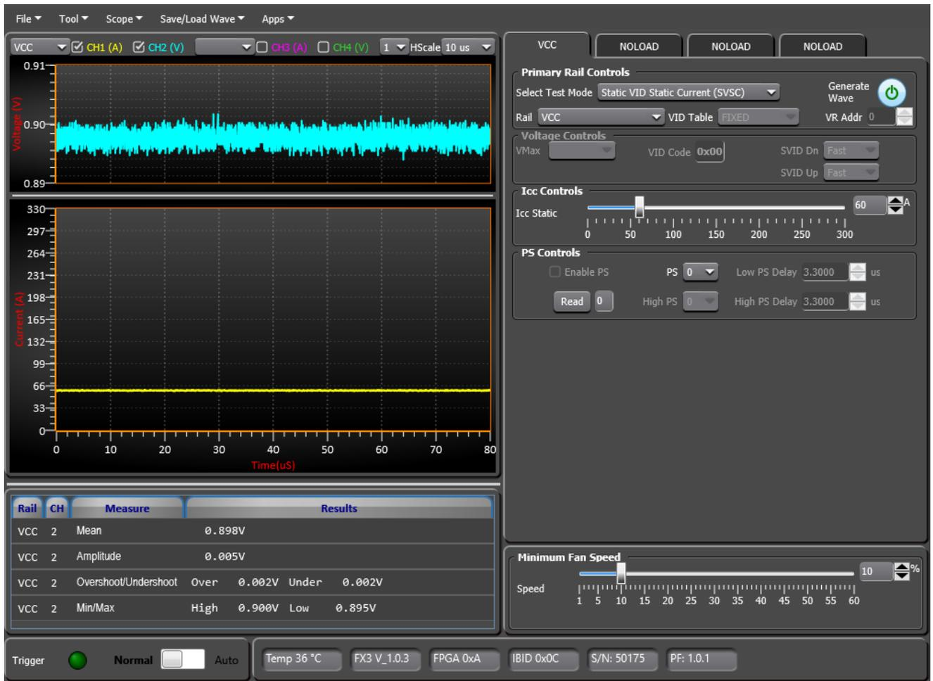
**Figure 4: Static Testing on EM2260 for Core Rail ( $I_{OUT} = 60\text{ A}$ )**
