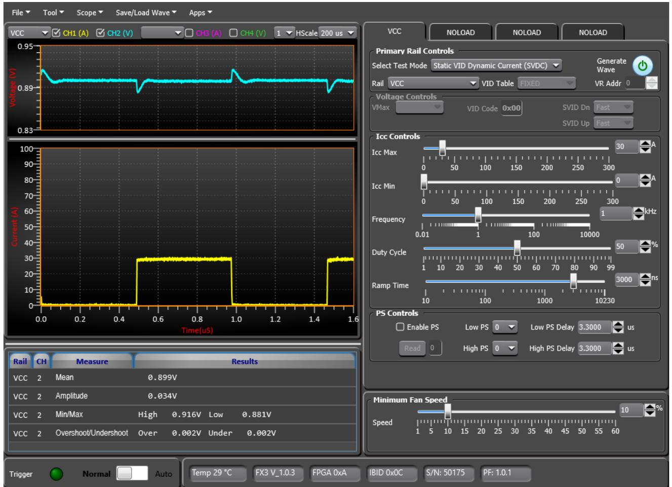
Figure 5: Dynamic Testing on EM2260 for Core Rail ( $I_{OUT}$  Load Step = 0-30 A)
