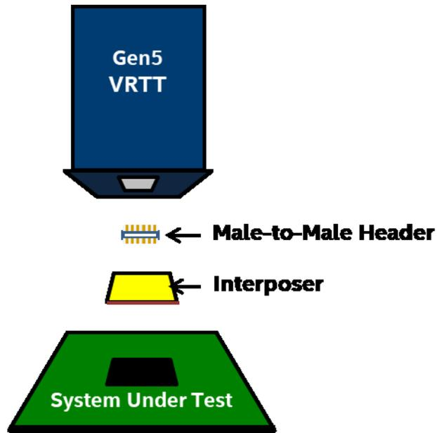
Figure 1: Test Setup Diagram
