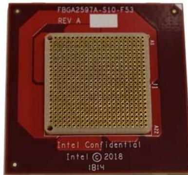
Figure 3: Gen5 Compatible Intel® Stratix® 10 MX FPGA Interposer
