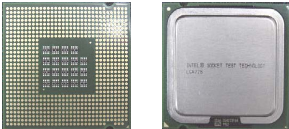
Figure 1 - Intel® Socket Test Technology for the LGA775 Socket—Test Chip
